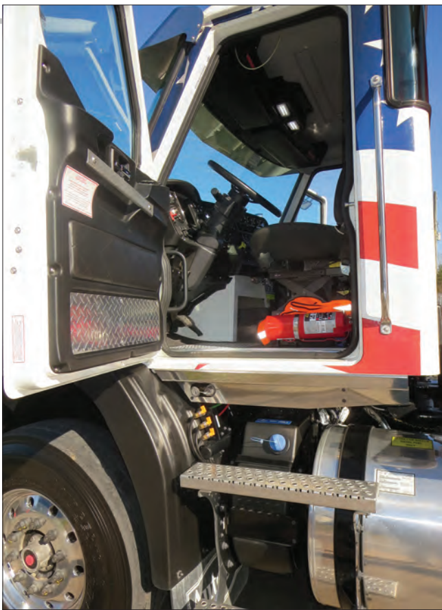
Three high steps carry a driver into the nicely appointed cab. Note the yellow switches under the door's front, for remotely draining air tanks, and rear corner windows that aid outward visibility. Tanks for fuel and diesel exhaust fluid are conveniently mounted on the left side, though they could go elsewhere.
