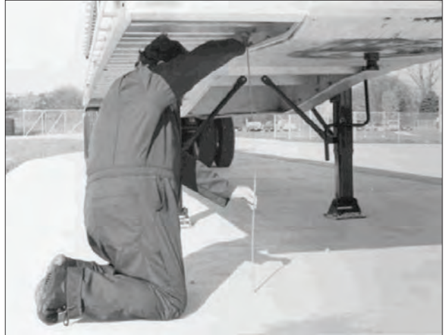
A technician measures the height of the upper coupler platform, and therefore the kingpin, prior to other work. Height is altered by adjusting the landing gear up or down. Trailer must be on level pavement for all alignment work.
