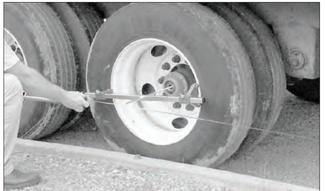
Wheel end extender brings the hub’s center out to where a tape measure can reach it while stretching from the trailer’s kingpin. It’s among the specialized tools needed to do a proper alignment.
